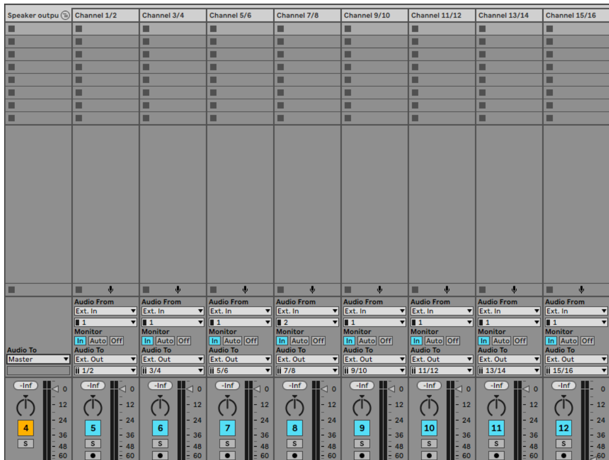
Figure 2: The correct setup of the 8 output tracks in an Ableton session for using Audiocanvas and Placer.
