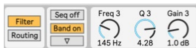
Figure 4: The frequency, Q and Gain dial for a band in the filter section.
